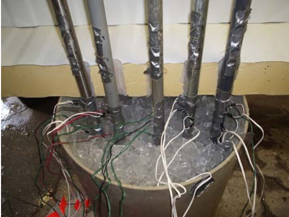
Figure 2: Conduits from left to right – SST, Schedule 80 PVC, aluminum, rigid steel, and PVC coated rigid steel
