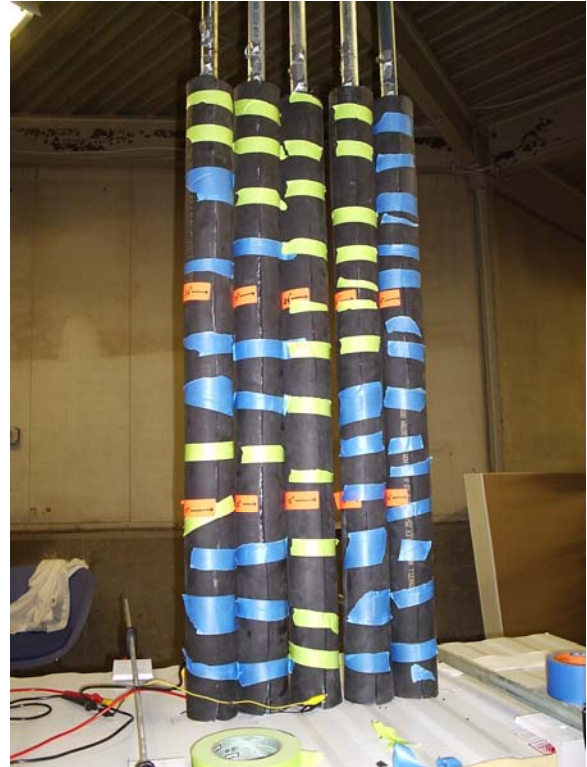
Figure 3: \frac{3}{4} " Insulation installed 36" above the insulated metal panel.
