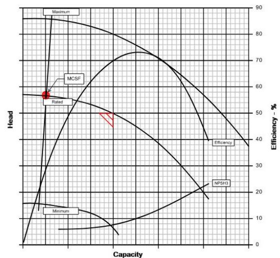
Example pump curve showing the Minimum Continuous Safe Flow (MCSF).
